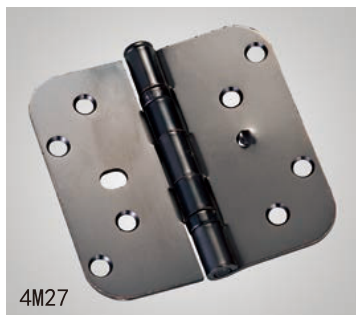
4M27 Residential Door Hinge 4" x 4" x 2.5mm-2BB
